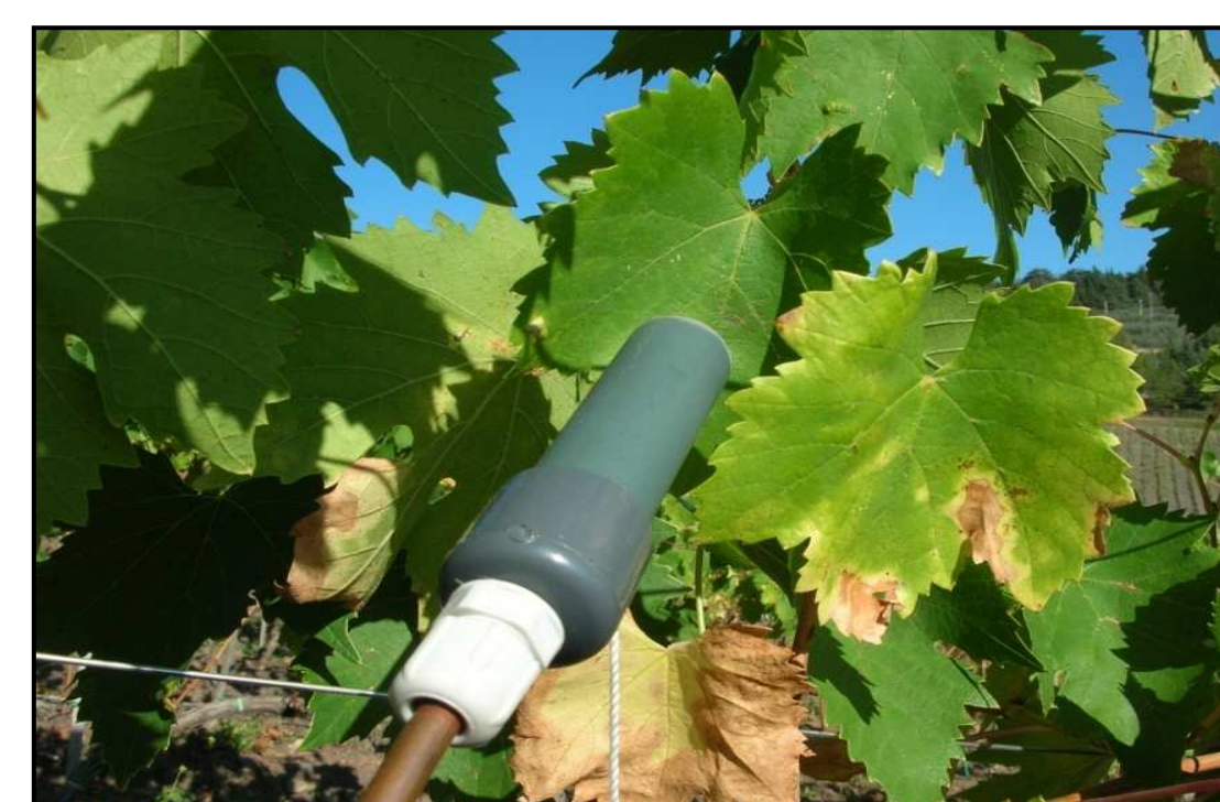
Fig.3 Air and leaf temperature sensors
